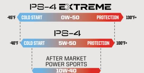
• Our best extreme high temp formulation, excellent for severe high temperatures and for racing, even at temps over 54°C.
